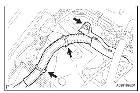
(d) Remove the 2 bolts and No. 1 oil reservoir bracket.
