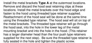
NOTE: The job of the plastic screw is expanding the legs of the retainer into the hole. The screw will not fully tighten. Stop threading the screw when it is flush with the head of the fastener.
