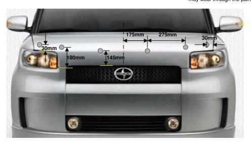
Open the hood of the vehicle. Peel and fold an anti-abrasion film pad in half over the edge of the hood, in the four (4) locations shown in illustration.
